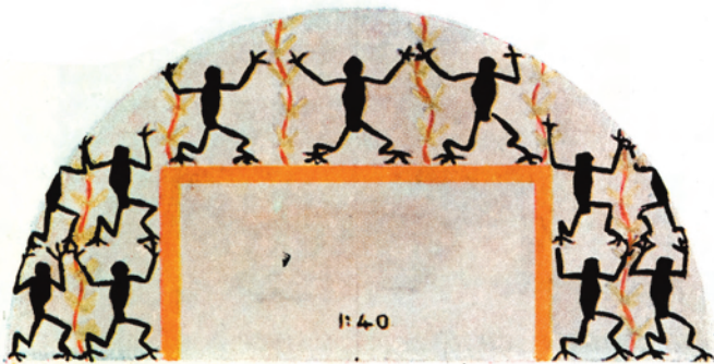
Grille for Nation's rooms in Guarany style, single motif taken from document. made of painted iron
